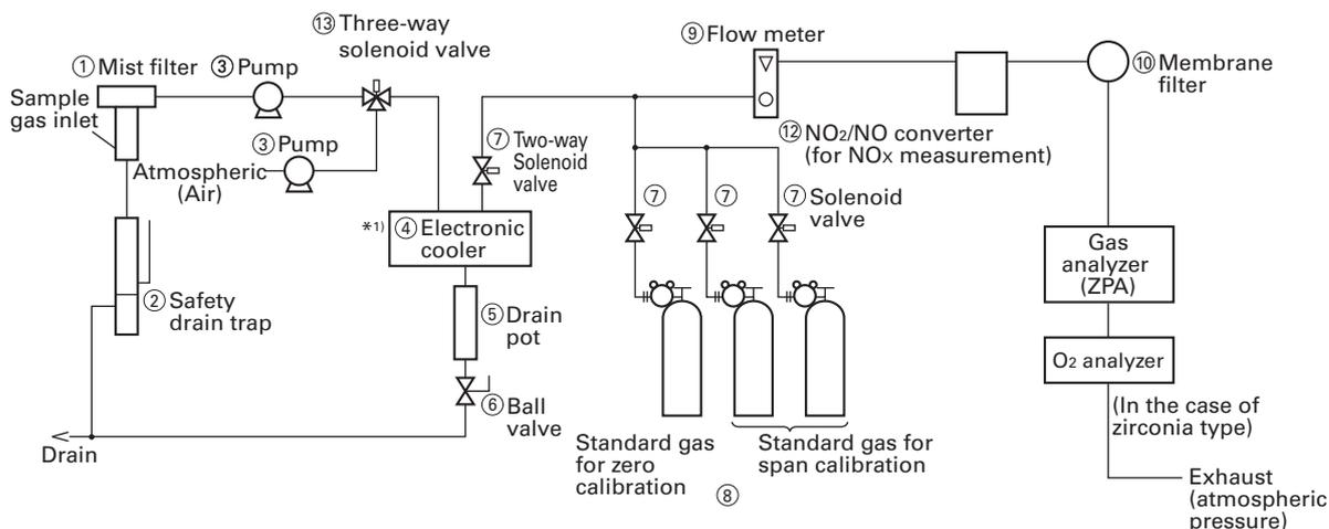
\*1) For NO, SO<sub>2</sub>, or 0–200 ppm range CO measurement, be sure to use an electronic cooler to keep the moisture content below the level saturated at 2°C.
